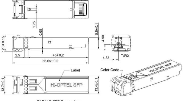
BI-DI LC SFP Transceiver (Unit: mm View:  $\bigcirc \oplus$ )
